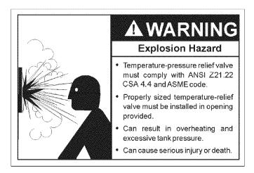
This heater is provided with a properly certified combination temperature - pressure relief valve by the manufacturer.
